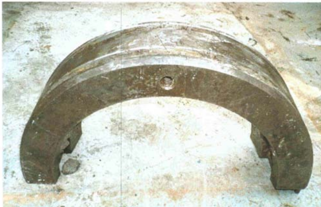
13 3/8" X 20" FMC wellhead casing slip segment weighing 35kg
